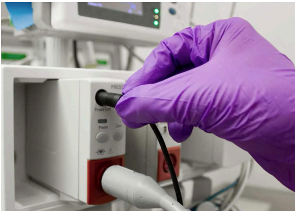
The Argos simply connects to the analog output of the blood pressure signal from a compatible multi-parameter monitor.
